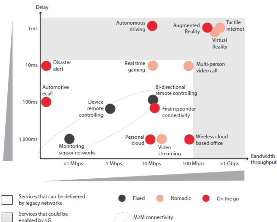
Figure 2.1.2. Potential 5G use cases: Bandwidth and latency requirements [3]
